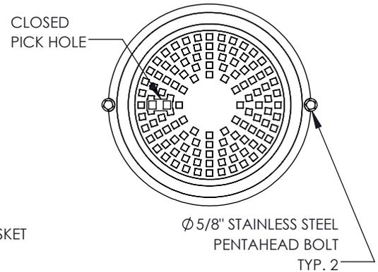
BOLT-DOWN WITH CLOSED PICK HOLE COVER
